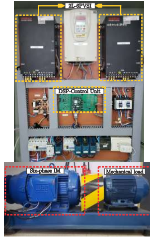
Figure 7. Test bench composed of the 2L-6PVSI, DSP unit control, six-phase IM and the mechanical load.
