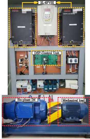
Fig. 7. Test bench composed of the 2L-6P VSI, DSP unit control, six-phase IM and the mechanical load.
