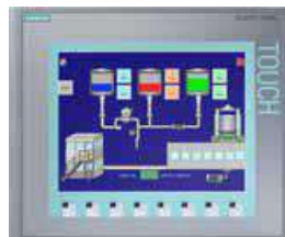
Figura 7. 13: HMI KTP 1000 Basic PN
